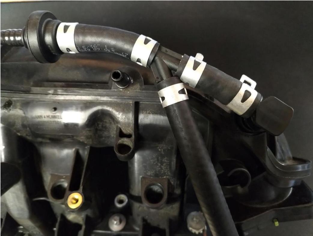
Note: The hose supplied with the kit should measure approximately 11". I measured an ideal length of 10.5" on my own intake manifold. Trim the hose if you find that it is too long.
