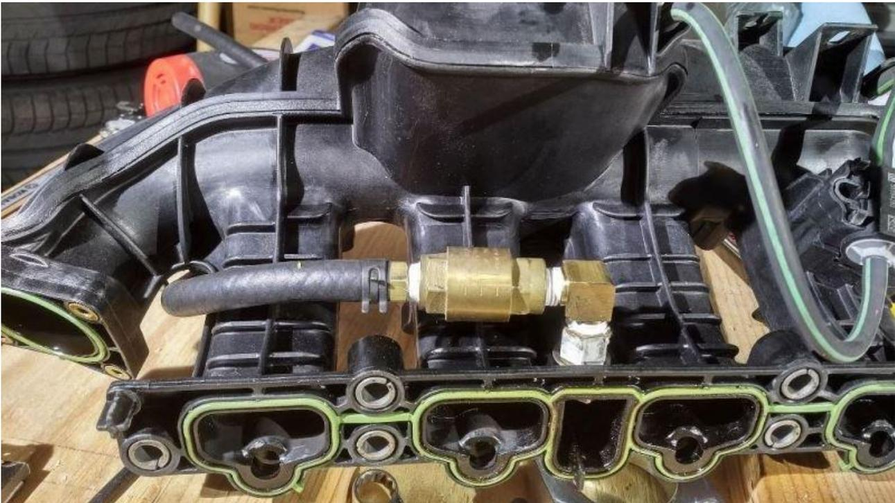
13. Attach the Y fitting to the EVAP purge line. Method 1 is to attach the Y fitting directly to the EVAP purge valve line. To do this, cut the EVAP purge valve line 2-1/4" away from the terminal, then trim 5/8" off of the other end (the check valve side). Hold the Y fitting in a vice, spray it with silicone spray, and slowly heat the nylon line while pressing down on the line firmly.
