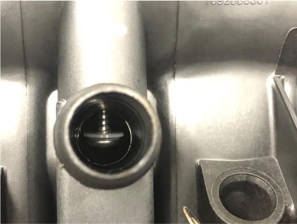
4. Place the washer over the screw, and liberally coat the screw thread with epoxy.
