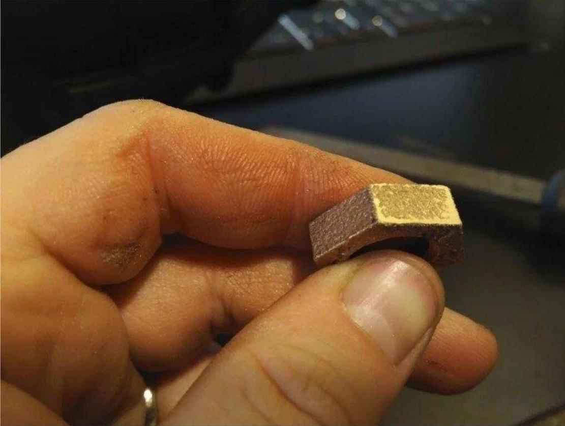
8. Fit another un-modified washer over the NTP adapter, and fit the adapter through the hole. Fit the nitrile gasket over the threads, followed by the washer you filed down.
