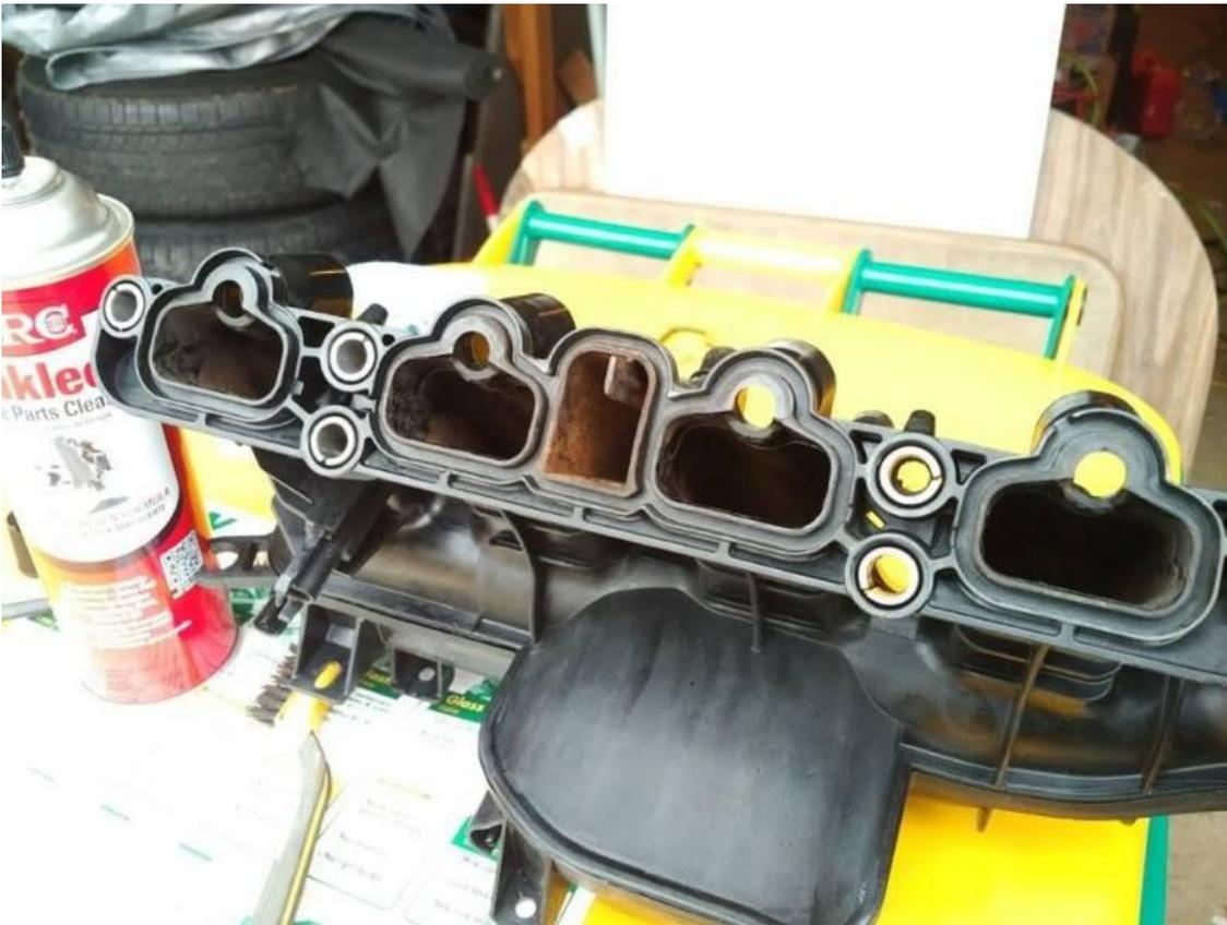
3. Below is where you will be installing the screw and washer. The idea is that if your check valve is missing that hole needs to be plugged up as it's creating a boost leak. First, drive the screw half way into the center hole for the check valve dry (without any epoxy) to start the thread, then back out.
