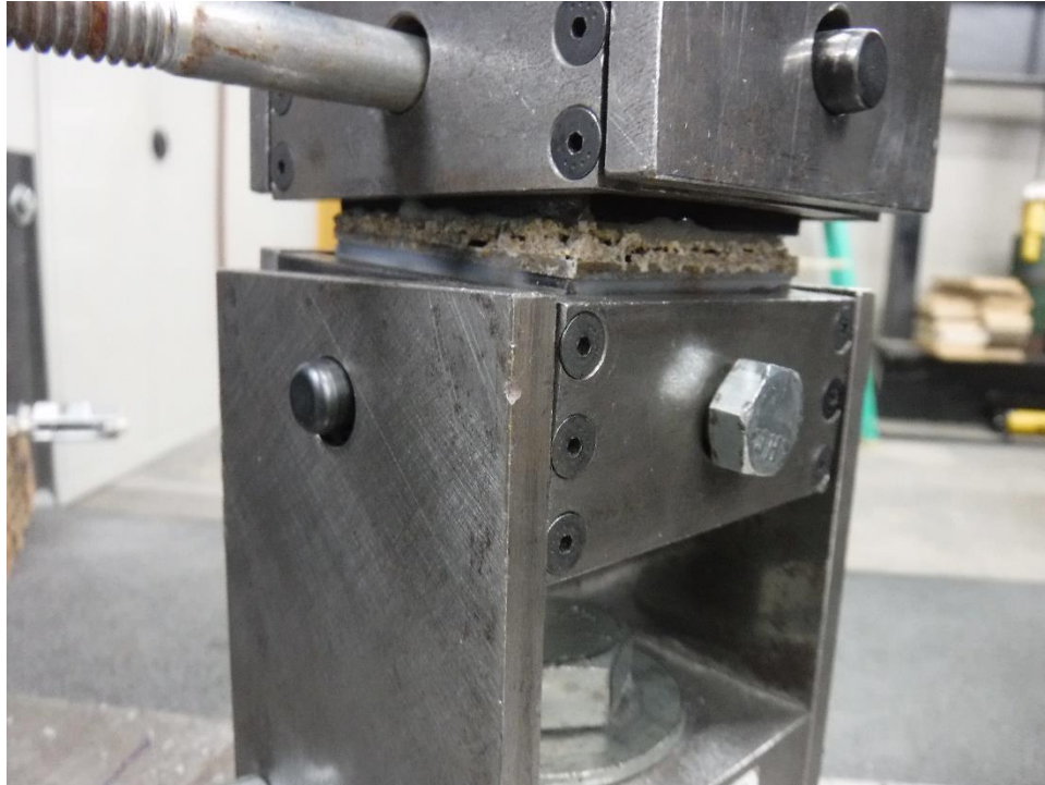
Photo No. 3 Cohesive Failure of F08 Corkshield During Testing (Metal)
