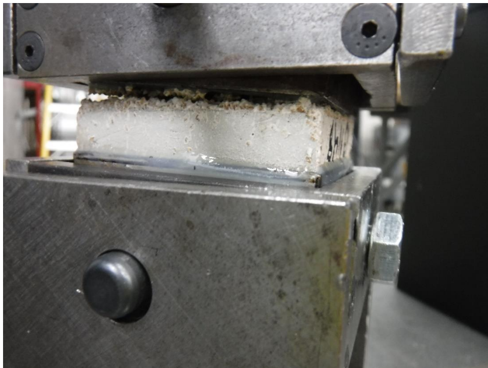
Photo No. 4 Cohesive Failure of F08 Corkshield During Testing (Stucco)
