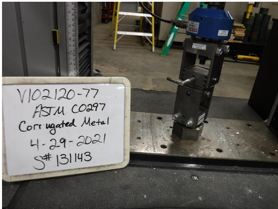
Photo No. 2 ASTM C297 Test Setup
