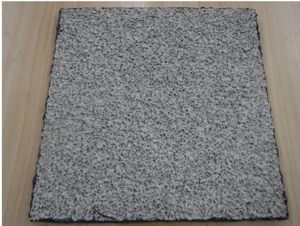
Photo No. 8 Specimens After Freeze-Thaw Cycling
