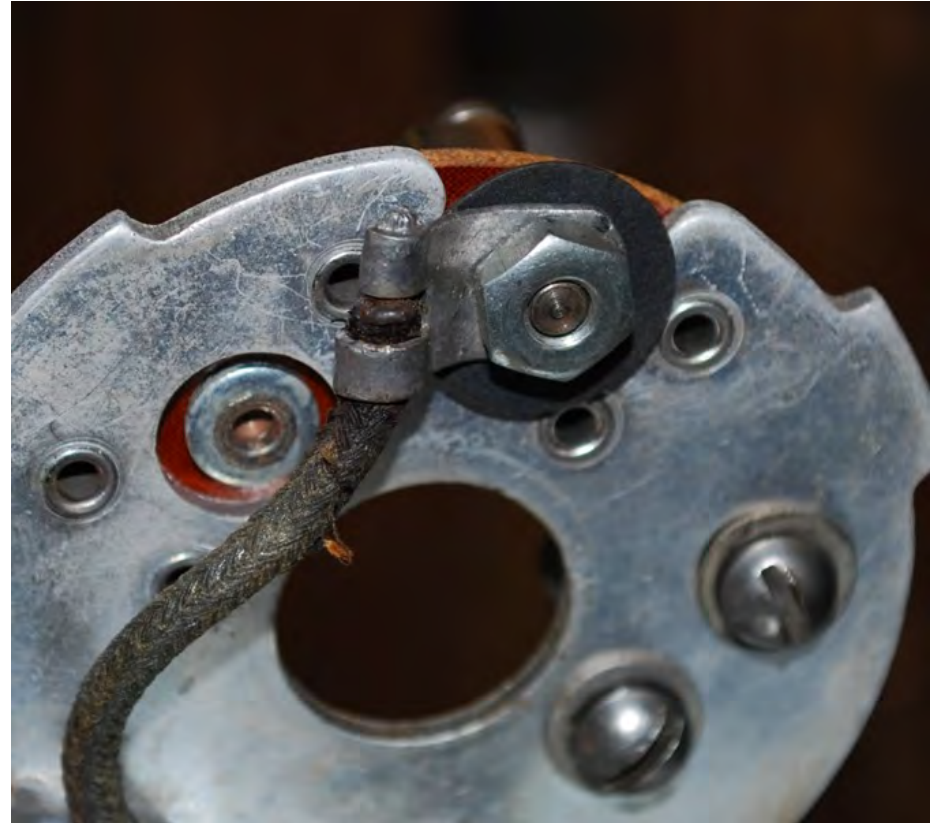
Lower plate wire to upper plate connection
