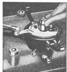
Fig. 24 (left). Distributor body and rotor replaced. Rotor arm is turned opposite No. 1 high-tension contact in distributor head.
