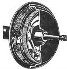
Fig. 51. Rear wheel brake showing the two-in-one brake drums.
