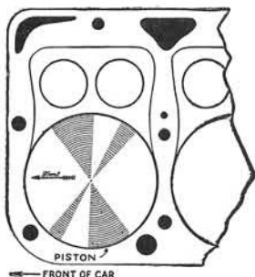
Fig. 58A. Markings on pistons. To eliminate any possibility of pistons being incorrectly assembled in an engine, the word "front" is placed beside the arrow, that is, stamped on top of the piston. When the piston is correctly assembled in the engine, the arrow will point toward the front of the car and the split in the skirt will be toward the left side of the engine (left and right side is always determined from driver's seat).
