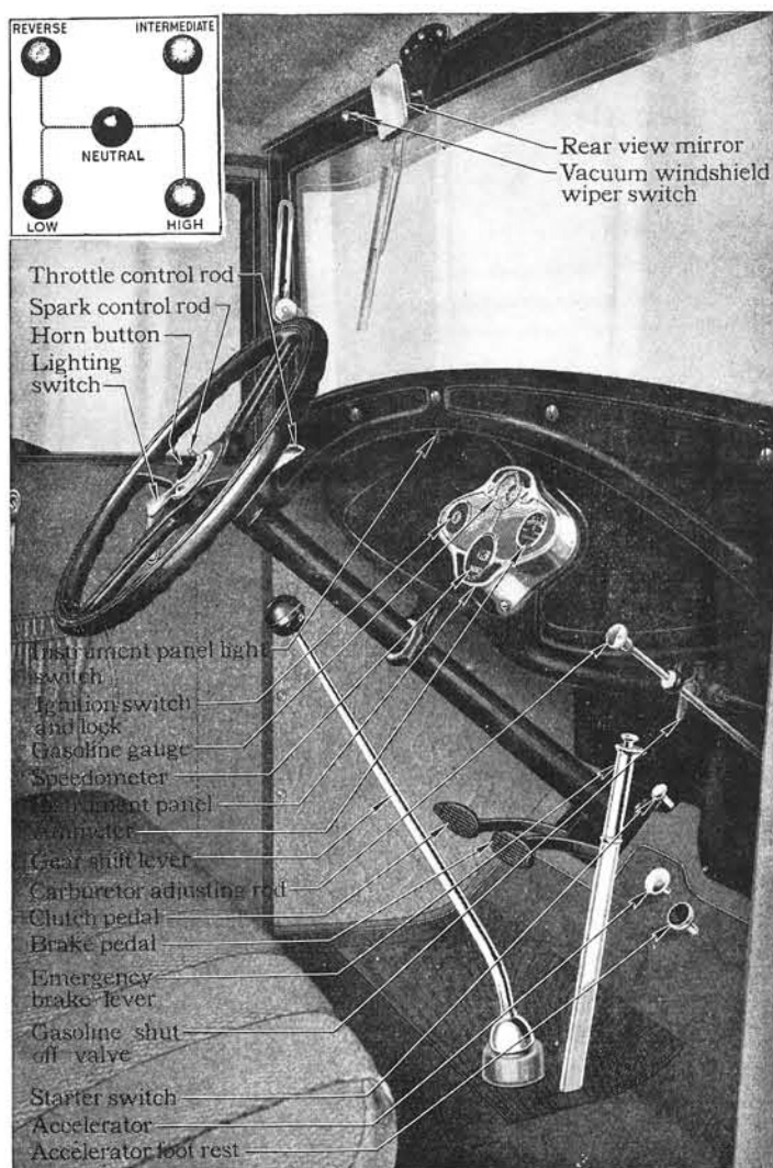
Fig. 1. Instruments and control levers of the model "A" Ford car. The gear shift is shown at the top, left corner.
