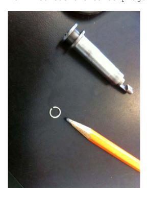
Magic Image Labeled CARB3: I removed the clip from the brass adjusting needle housing. This clip is supposed to be removed before installation. This is a beginner's curse used for shipping purposes only.
