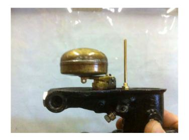
Magic image labeled photo.JPG: I adjusted the float per our Caribbean Factory specs. It is now parallel to the carb housing at exactly 1" when valve is closed. I also exorcized the dimple from the float located at the point of contact to the float valve. Dimples or holes worn in over time can kink the valve off center and not seat properly. I believe there is magic image of this in the FORD BARNYARD under leaking carburetor tips explaining the exact same curse I found on your float.
