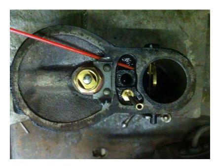
Magic Image Labeled CARB2: The over flow or flood hole was completely plugged. This is where your carb is supposed to leak when the float valve sticks open. I believe it also acts as a breather to equalize pressure inside the carb bowl. When this hole is plugged, I'm sure this could have created unwanted pressure
