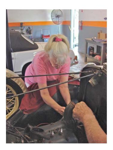
During the following week, I met with the Davis' to prep and paint the front end and engine in preparation for the installation of the radiator. Russ Gagliano took the radiator to one of his vendors and had the radiator cleaned and repaired. Then Russ painted the radiator and delivered it to Roberto's garage for our June 9th workshop. While I was at Roberto's, we changed the oil and greased the car, and checked the air in the tires.
