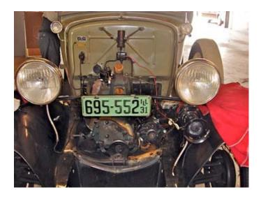
We rebuilt and replaced the water pump, the distributor and the carburetor. We installed new spark plugs and reset the timing. We also replaced the wheel that was corroded. We made a list of parts that would be needed and I ordered them from Phane Jones who rushed them out to me so we would have everything for the next workshop.
