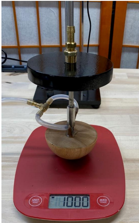
A fixed gravity load of 10 Newtons is applied to the probe
