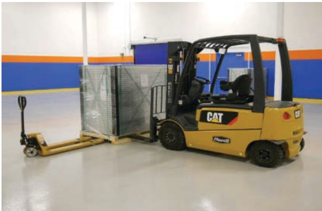
Fig. 9: How to handle the packaging - When using a forklift, please ensure the forks go all the way through pallet. The fork length should be a minimum of 1800 mm
