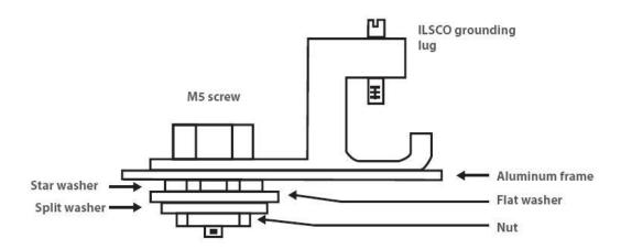
For module with Φ5.1mm grounding holes
