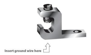
Attach a separate ground wire to grounding holes on modules frame with a self tapping screw. Module frame is provided with grounding holes. Stainless-steel bolts, with nuts, washers, and locks washers, are recommended for module grounding. The ground wire should be at least the same size as the electrical conductors, ground wires greater than 10AWG is recommended.
