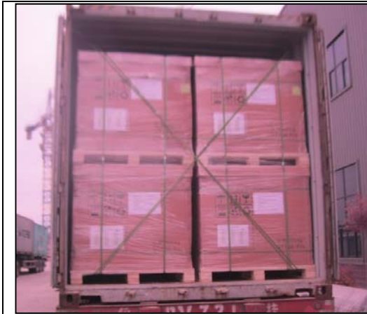
Step five: Loading into container and fixing with PE belt
