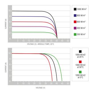
\*STC: (Standard Test Condition) Irradiance 1000W/m²; Module Temperature 25°C; Air Mass 1.5
