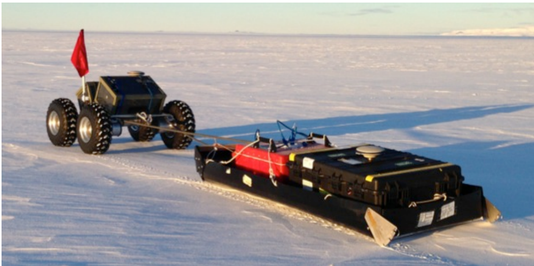
Figure 3. Yeti with a GPR sled in the McMurdo Shear Zone. The black case housed the radar controller, batteries, and GPS receiver and supported the GPS antenna ( white disk ). The orange 200 MHz antenna and smaller 400 MHz antenna (not visible) mounted in front of the black case. The black polyethylene sled included two steel rudders to reduce yaw motions. The sled and GPR equipment weighed 74 kg. Yeti's radio antenna carried a red flag; its GPS antenna mounted on the opposite side in front of the battery box.
