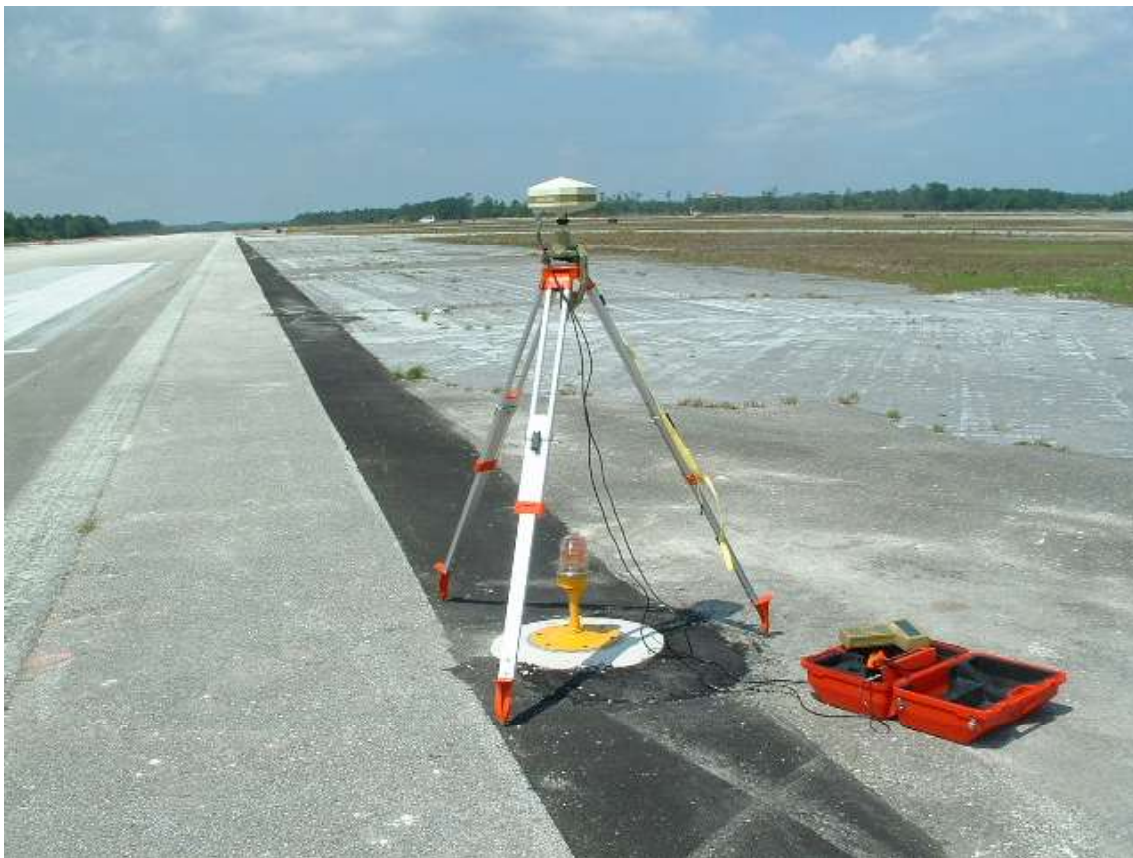
Figure 2-3. Airfield NAVAID positioning using Fast-Static GPS methods
