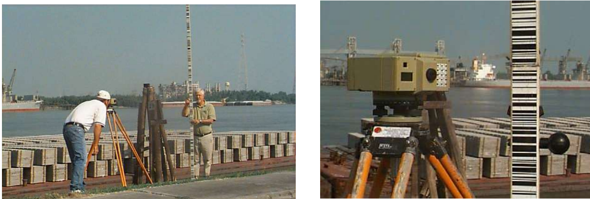
Figure 3-26. Digital Bar Code Level--Wild NA2 (New Orleans District)
