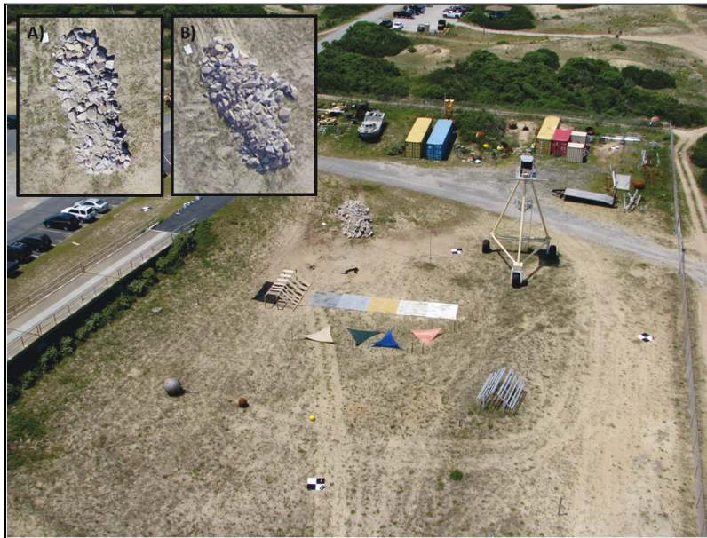
Figure 3-6. Image of target pad area and UAS evaluation targets. Camera position is east of the target pad, oriented west. Inset: Image of (A) intact and (B) destroyed mock jetty.
