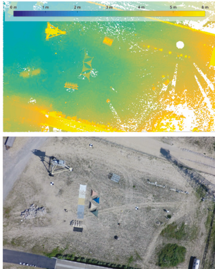
Figure 3-7. Example point cloud in plan view (top) and near nadir UAS image (bottom) of target pad area. Point cloud scans performed 26 June 2017. NAVD88 1 elevation plotted in point cloud; color is saturated with a maximum of 6 m to highlight low-elevation targets. Imagery from CHL X8+.
