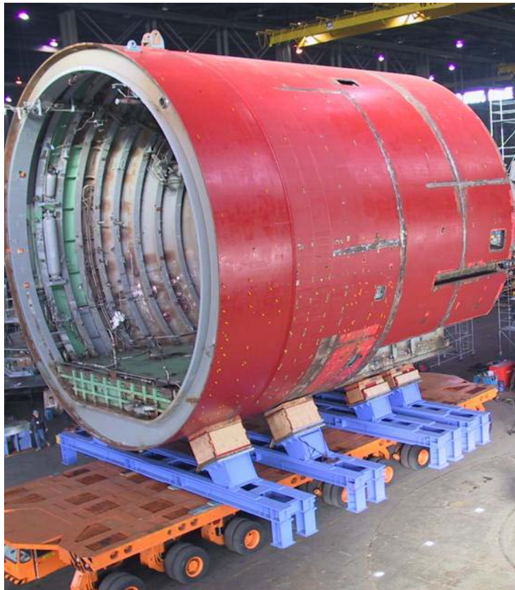
Figure 10.1 A hull section of the SSN-21 class shown during assembly. The transvers frames are shown clearly at left (the hull is a ring stiffened cylinder)
