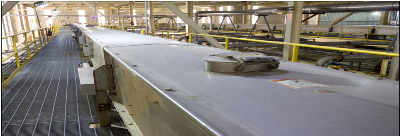
Figure III.3. Enclosed Belt Conveyor
