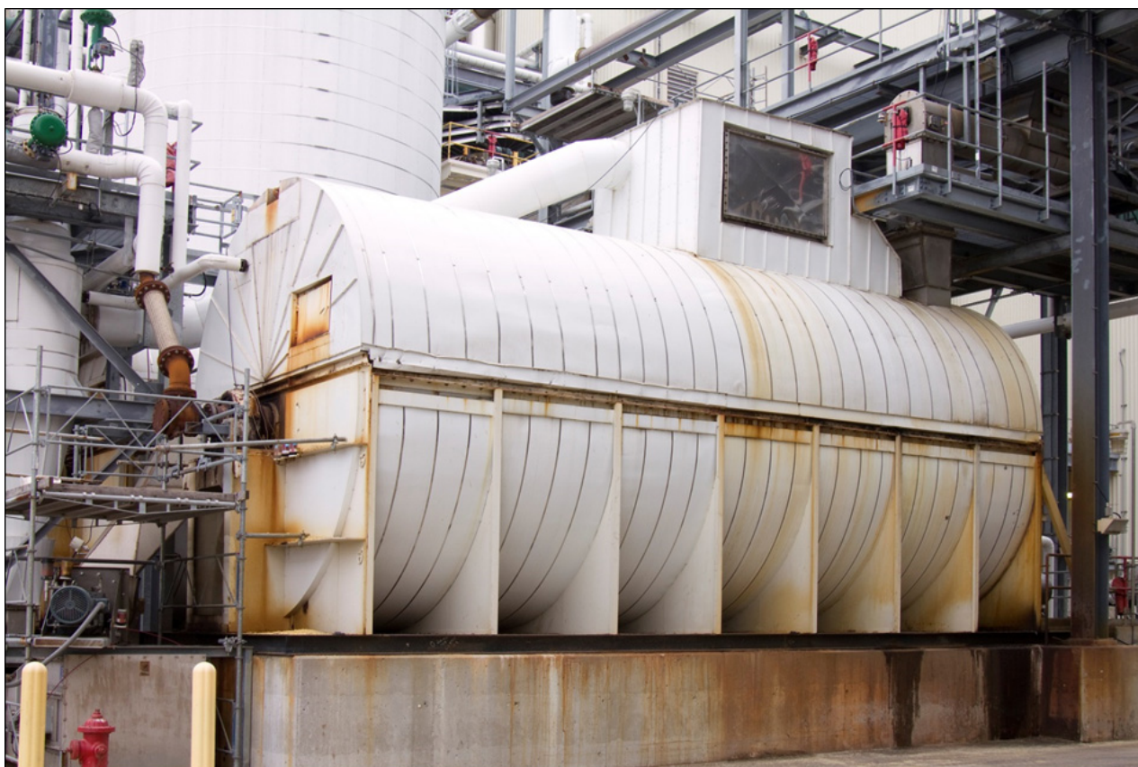
Figure II.17. A Rotary Drum Dryer
