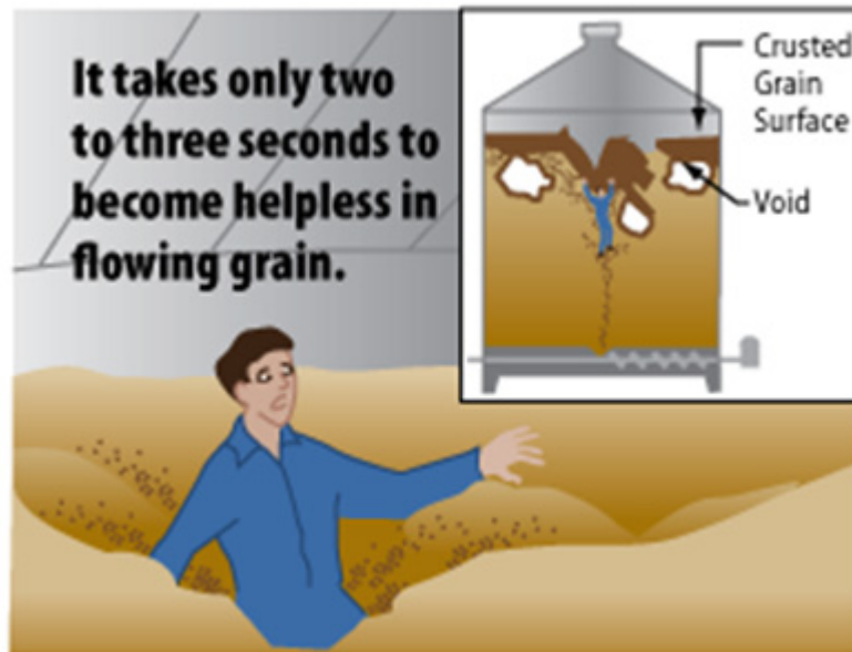
Figure III.5 Image of a Grain Engulfment Hazard
