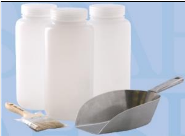
Figure VII-1: Sampling Kit: 1 Liter Sample Collection Bottles, Metal (Aluminum) Scoop, and a Natural Fiber Brush. (Source: OSHA SLTC)
