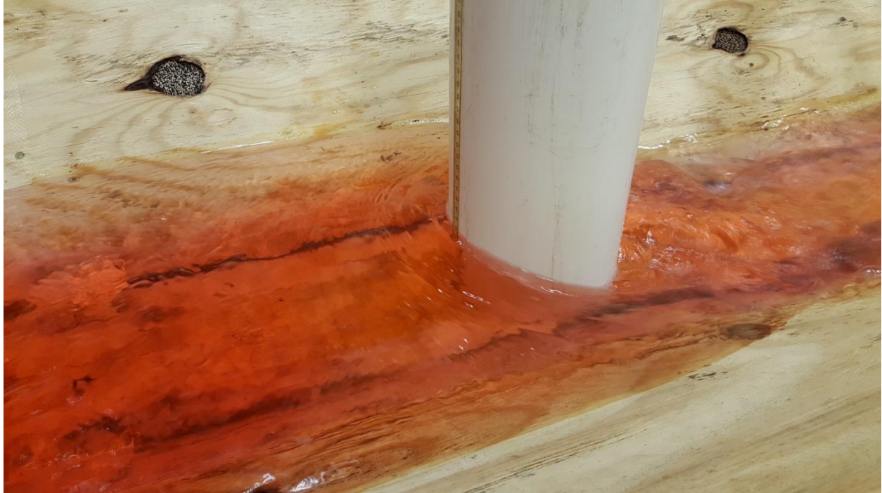
Figure 23. Trapezoidal flume testing in the lab with critical flow.
