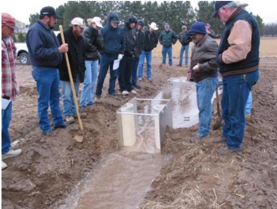
Figure 17. S-M rectangular flume installed in an unlined ditch in southern New Mexico.
