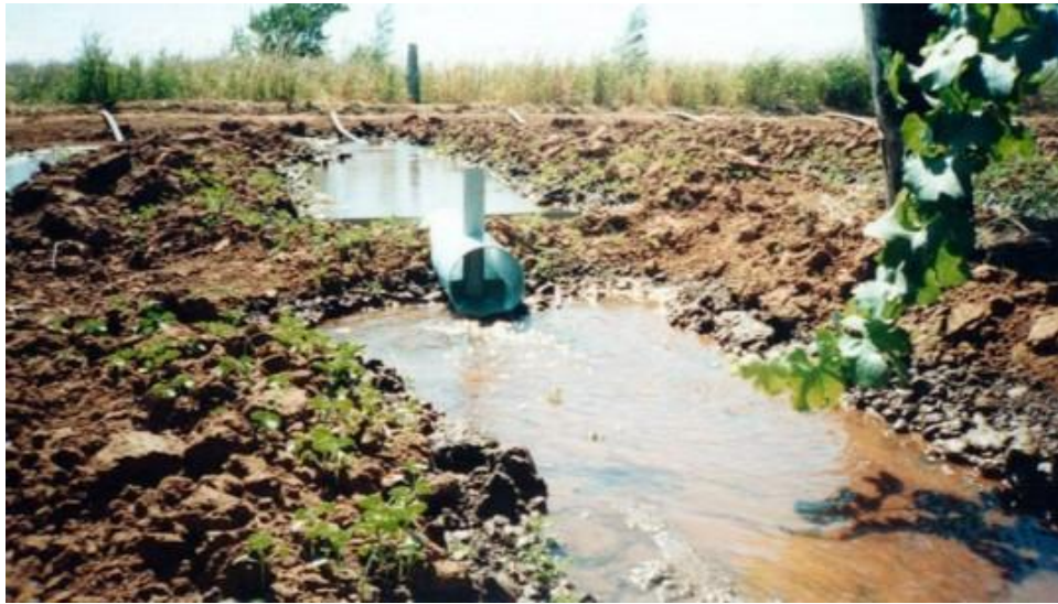
Figure 9. Circular flume installed in a vineyard in Australia.
