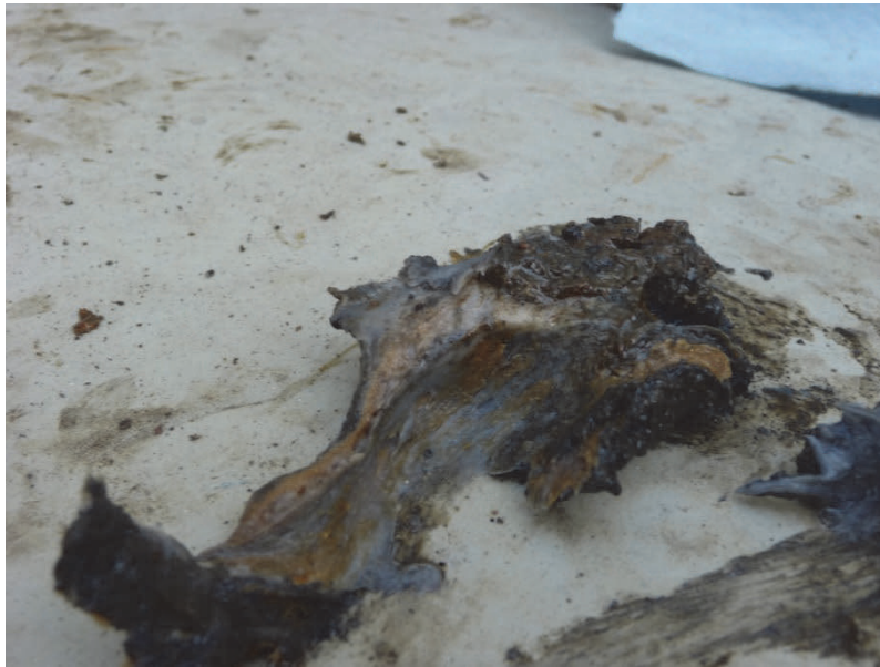
Figure 2.12. Grease with biological growth at John Day lock when anchor head was removed (Ebeling et al. 2013).
