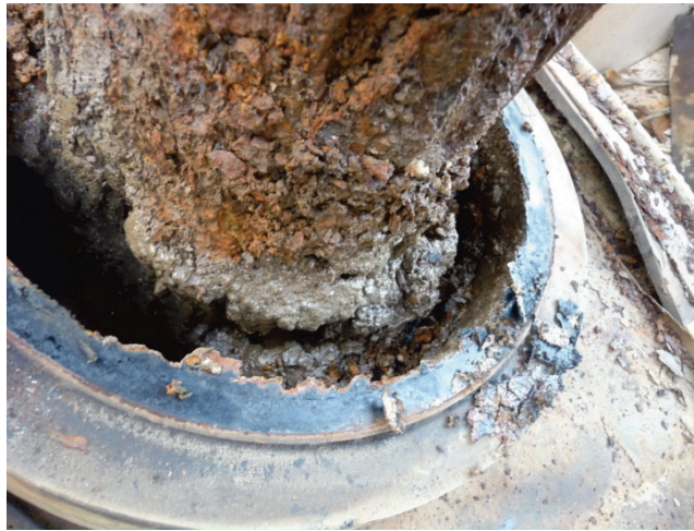
Figure 2.10. Example of accelerated corrosion due to biological agents in existing grease (Ebeling et al. 2013).
