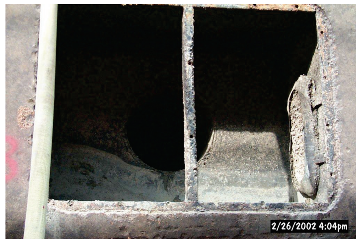
Figure 2.4. Example of anode protecting ship's hull (cathode). This is the U.S. Army Corps of Engineers Dredge Jadwin in dry dock. Note the partially consumed anode (to the right) at the entrance of the engine cooling water intake.
