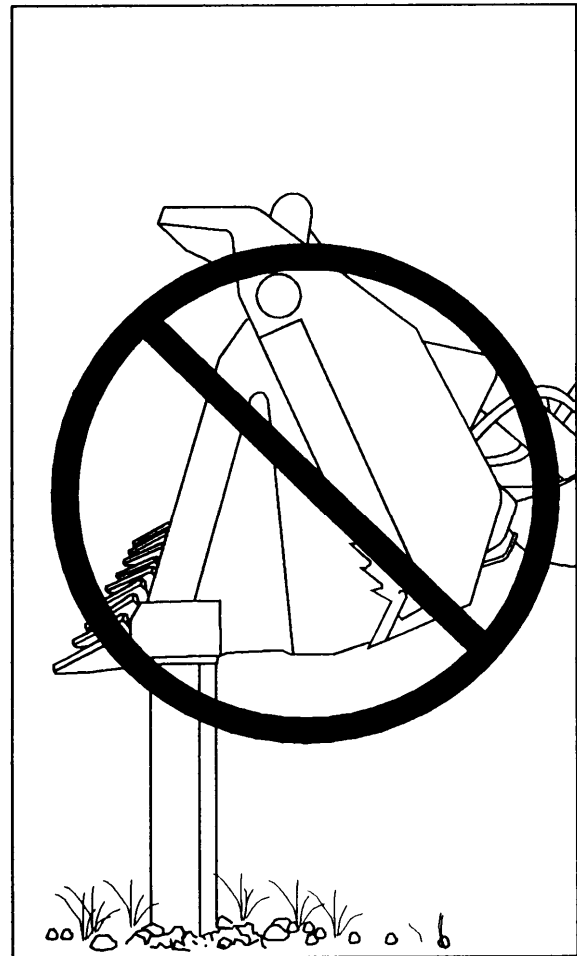
Figure 9-34.-Using the bottom of the clamshell as a pile driver.
