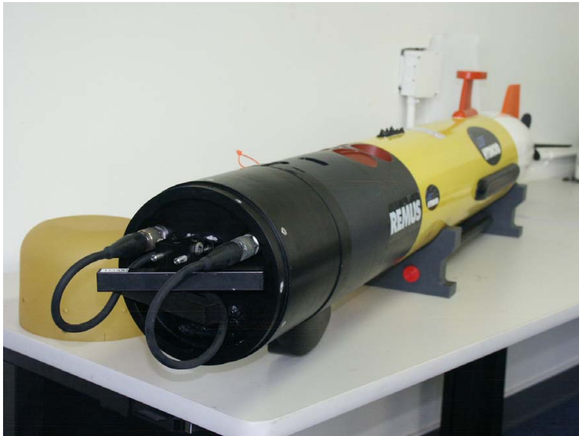
Figure 7. Naval Postgraduate School REMUS AUV with BLUEVIEW FLS. Note the nose cone is removed, and the transducers are in the horizontal configuration.
