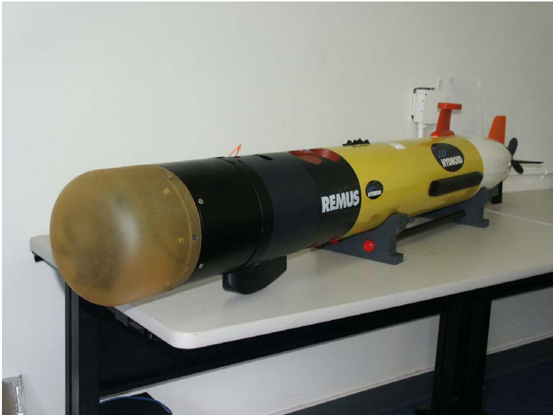
Figure 6. Naval Postgraduate School REMUS AUV with BLUEVIEW FLS
