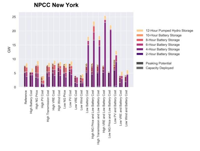
Figure A-15. Economic storage deployment and peaking capacity potential of storage in 2050 in all resource sensitivity scenarios in the NPCC New York zone (Figure A-7)
