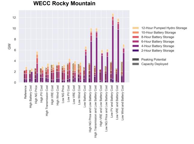
Figure A-25. Economic storage deployment and peaking capacity potential of storage in 2050 in all resource sensitivity scenarios in the WECC Rocky Mountain zone (Figure A-7)
