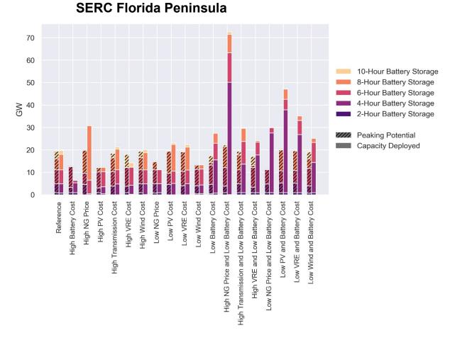
Figure A-18. Economic storage deployment and peaking capacity potential of storage in 2050 in all resource sensitivity scenarios in the SERC Florida Peninsula zone (Figure A-7)
