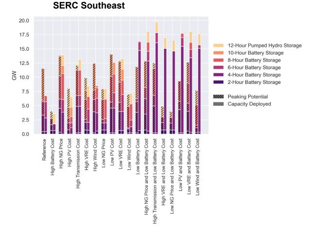
Figure A-20. Economic storage deployment and peaking capacity potential of storage in 2050 in all resource sensitivity scenarios in the SERC Southeast zone (Figure A-7)
