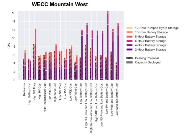
Figure A-23. Economic storage deployment and peaking capacity potential of storage in 2050 in all resource sensitivity scenarios in the WECC Mountain West zone (Figure A-7)
