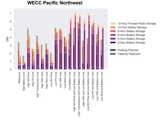
Figure A-24. Economic storage deployment and peaking capacity potential of storage in 2050 in all resource sensitivity scenarios in the WECC Pacific Northwest zone (Figure A-7)
