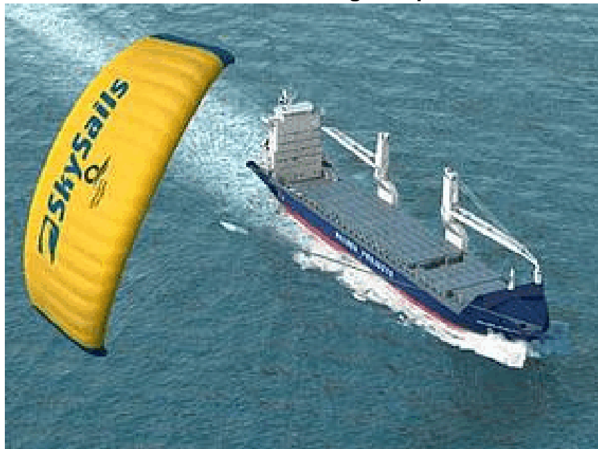
Figure 9. SkySails Concept Applied to Commercial Cargo Ship
