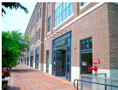
Figure 9.12. A pedestrian promenade serving ground-floor tenant spaces with no fire apparatus access. Below the red control valve is an exterior FHC.
