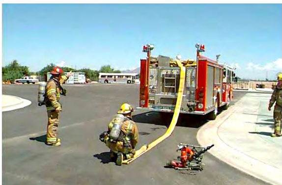
Figure 4.12. A pumper performing a reverse hose lay from a fire scene towards a hydrant. Once the hose lay is completed, the pumper will feed water through the hose line to the portable master stream device shown on the lower right.
