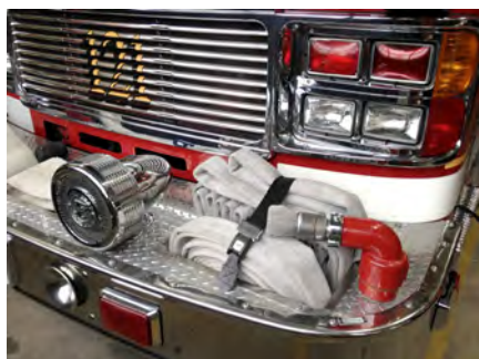
Figure 2.5. A preconnected hose line in the front bumper of a pumper. The hose is connected to the red pump discharge outlet on the right and a nozzle is connected to the other end of the hose.
