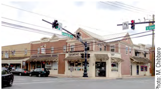
Figure 11.6. This building has multiple tenants with different addresses fronting on two streets. Strobes outside each exterior tenant entry door indicate the tenant where an alarm originates.
