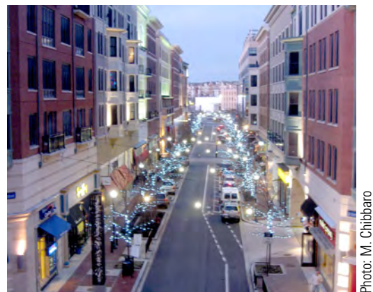
Figure 3.7. Lights strung across this street preclude the use of aerial ladders and limit the use of portable ladders.
