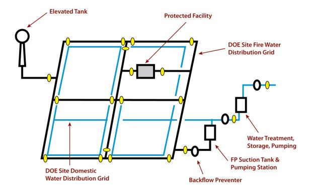
Similar to Arrangement 2, this arrangement should not be utilized for SC applications, but is used for general purpose fire protection and may be used for SS applications, if requirements for reliability, QA, and safe operation are met. The reason the system is not to be used in SC applications is that, even though the system is under DOE control, it is not under the facility's control. Thus having an additional backup system that is under the facility's control is prudent.
