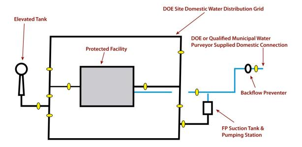
This arrangement could be utilized for SS applications, if conditions specified in A.3.2 and A.3.3 of Appendix A are met. If the supplied system (e.g., wet pipe sprinkler) needs to operate in a seismic event (e.g., to mitigate a seismically-induced fire), the supply system shall be qualified to the same level as the supplied system.
