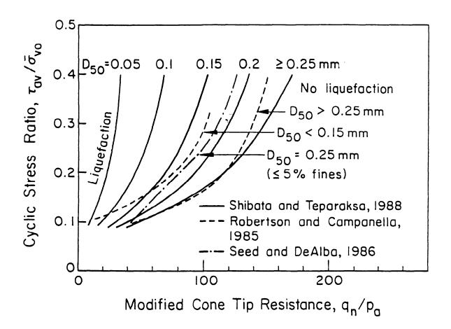
Figure 7. Liquefaction resistance with CPT values. from Shibata and Teparaksa (1988)
