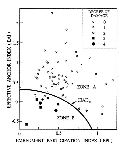
Figure 11. Sheet pile wall design chart. from Gazetas and Dakoulas, (1990) sponsored by National Science Foundation.
