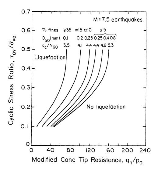
Figure 6. Liquefaction resistance with CPT values. from Seed and de Alba (1986)
