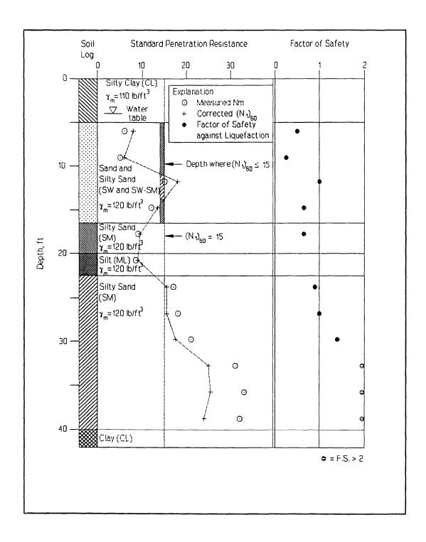
Figure 12. Boring log for example case.
