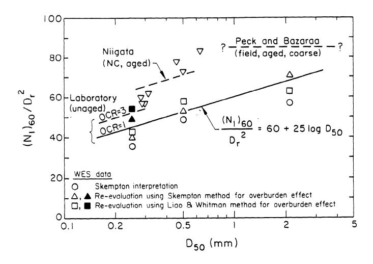
Figure 3. Particle size effect on blow count for sands. from Kulhawy and Mayne (1990), EPRI EL6800
