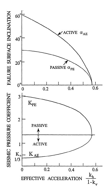
Figure 10. Failure surface inclination and pressure coefficients. from Gazetas and Dakoulas, (1990) sponsored by National Science Foundation.
