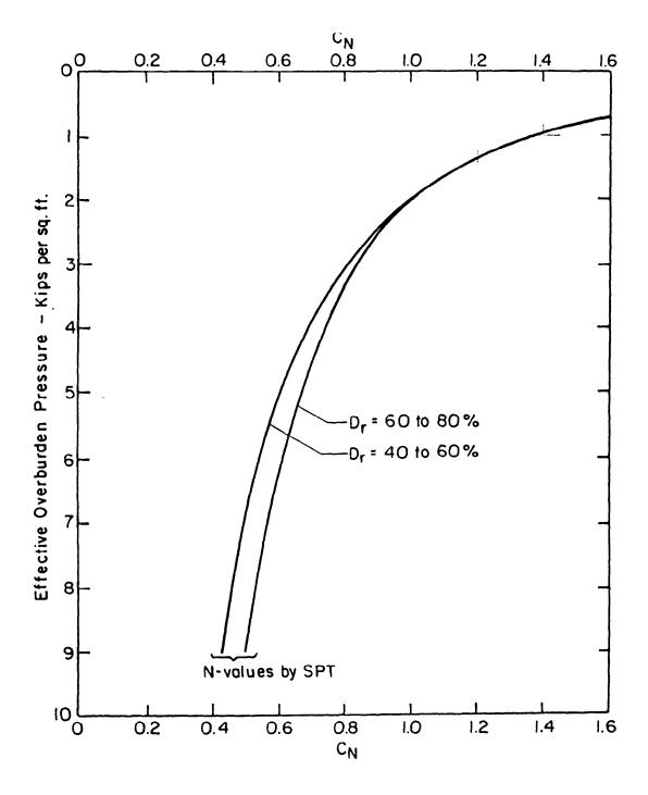
Figure 13. Effect of overburden on  $C_N$ .
