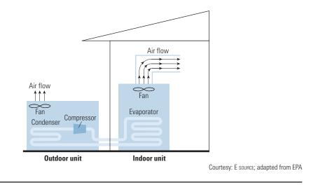
mode, the cooling system operates in reverse, extracting heat from the outside air and using it to provide space heating. Air-source heat pump systems range in size from about 1.5 to 25 tons. High-efficiency air-source heat pumps have an EER as high as 11.5 and a COP for heating as high as 3.6.
