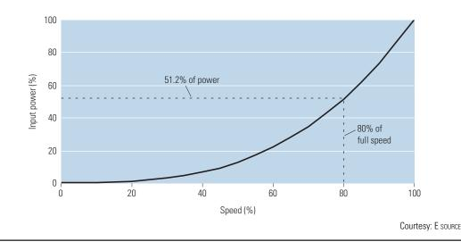
A VSD is not a motor; it is an electronic device that varies the speed of a motor by changing the frequency of the electrical power between 0 and 60 Hertz. The EPA study "Variable Air Volume Systems Maximize Energy Efficiency and Profits" showed that VSDs can greatly reduce the energy used by the same fan operating under similar airflow volumes and static pressure conditions. Overall, the study indicated that VSDs provided an average energy savings of 52 percent.
