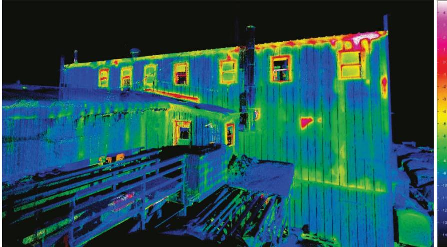
Figure 15. Southeast face of Biolab. The far right of the roofline shows significant heat loss along the roofline soffit. There is degradation of insulation below upper windows, possibly due to water leaking. The ceiling of the ground level and floor of the second level has heat loss along the exterior. A hot spot is visible to the right of the kitchen exhaust vent. Temperature scale:  $-15^{\circ}\text{C}$  to  $5^{\circ}\text{C}$ .
