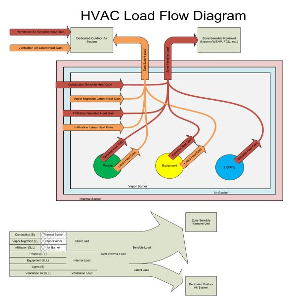
The HVAC Load Flow Diagram shows the components of HVAC load that are typically considered in an HVAC System Analysis. <u>Per this UFC</u>, the Dedicated Outdoor Air System (DOAS) should handle the latent loads for both the Ventilation Air and the Zone. The DOAS is typically a stand-alone, constant-
