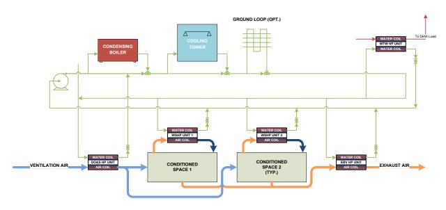
Energy Recovery Loop with separate DOAS and Exhaust ERV
