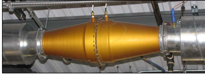
Figure 3. Laminar flow element used to measure airflow rates out of HPWHs
