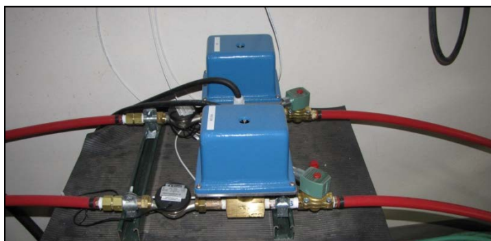
Figure 7. Outlet turbine flow meters, proportioning valves, and solenoid valves used to control outlet flow rate and draws
