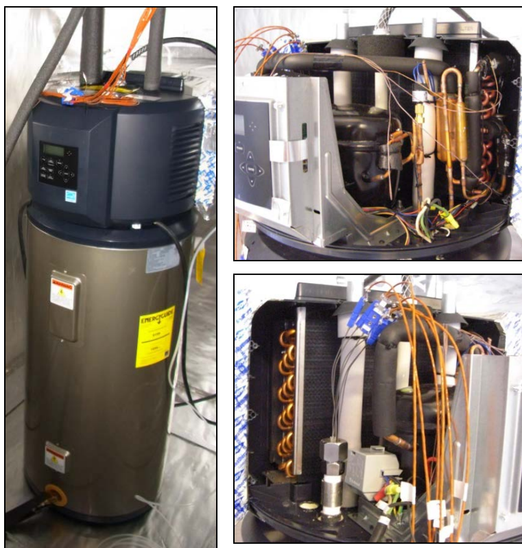
Figure 14. Unit B in the test plenum (left) and the instrumented heat pump components (right)
