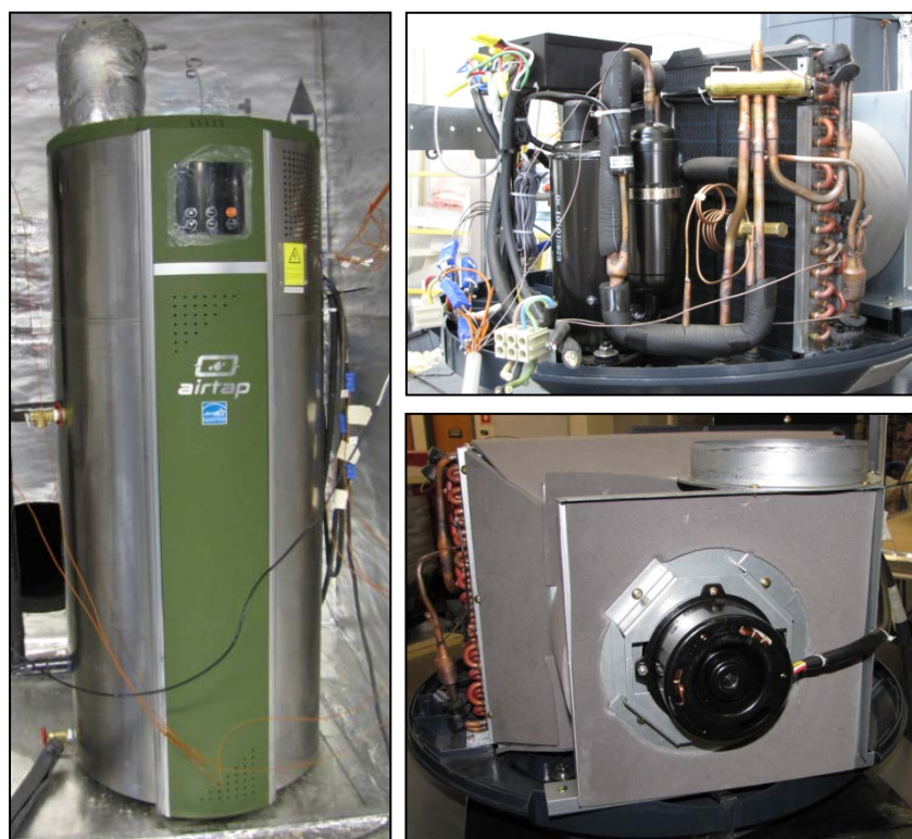
Figure 32. Unit E installed in test plenum (left). Some of the refrigerant system is shown (upper right), along with the blower that is designed to connect to a 6 in. duct (lower right)
