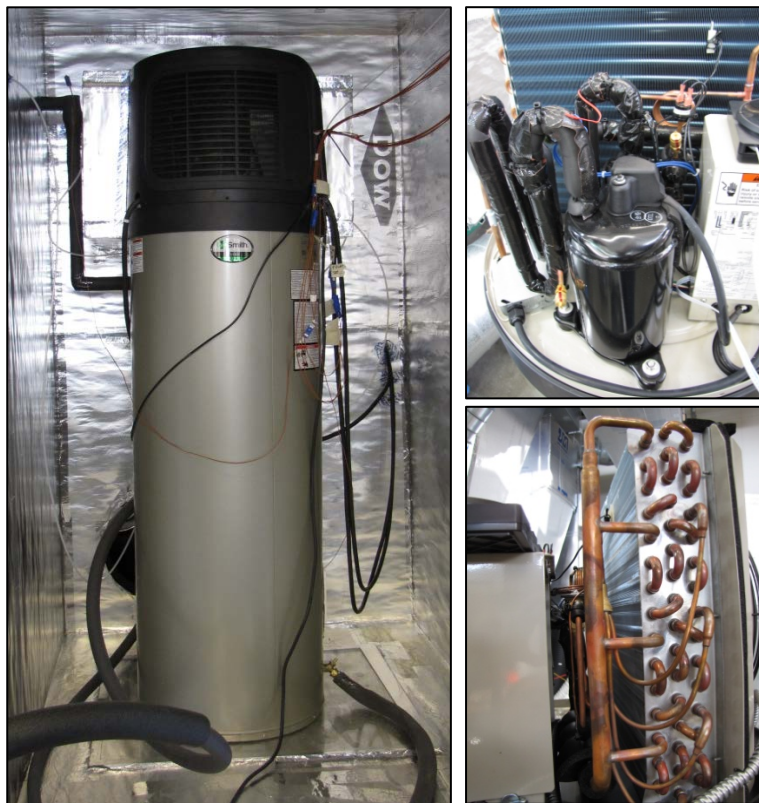
Figure 8. Unit A 80 gallon HPWH installed in test plenum (left). A close-up of the compressor and refrigerant system in Unit A (upper right) and a side view of the evaporator coils and heat exchanger (lower right).
