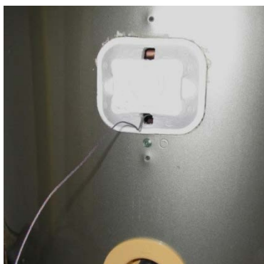
Figure 3. The insulation is replaced and the TC wire is directed through a hole in the insulation.
