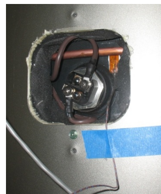
Figure 20. Surface-mounted TC at the lower tank surface
