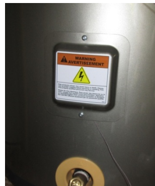
Figure 4. The cover is replaced, with the lower screw not fully tightened to give TC wire clearance.
