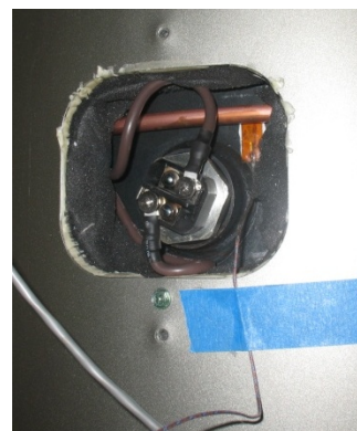
Figure 20. Surface-mounted TC at the lower tank surface
