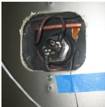
Figure 2. Surface-mounted TC is secured while the epoxy cures.
