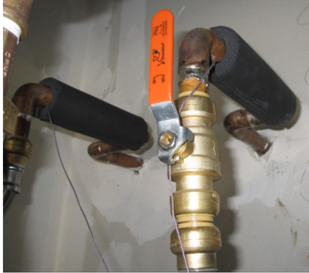
Figure 1. Pipe insulation covers the surface-mounted TCs on the inlet and outlet water pipes
