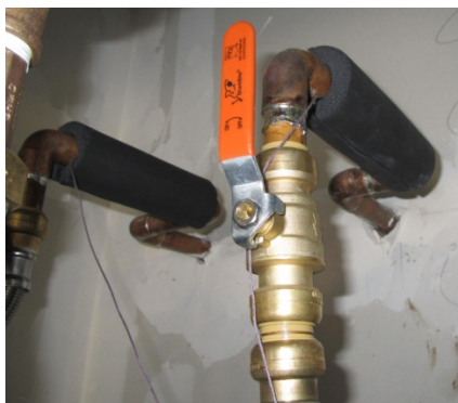
Figure 21. Pipe insulation covering the surface-mounted TCs on the inlet and outlet water pipes
