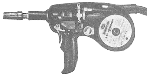
Figure 8-27.—GMA welding torch with wire feed motor and wire spool inside.
