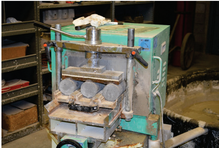
Figure 3.9. Marui Hi-Kenma end grinder.
