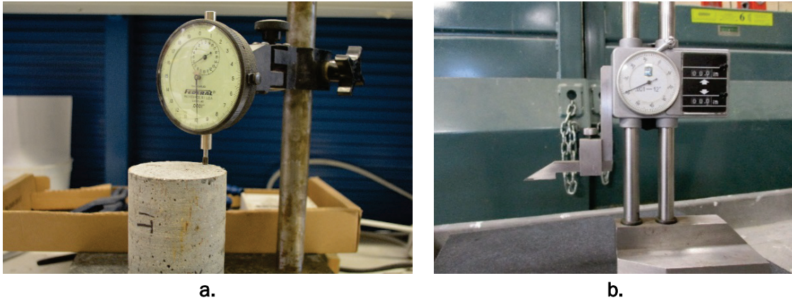
Figure 3.10. Gauges for measuring the deviation from parallel: a. ERDC, and b. Michigan Tech.
