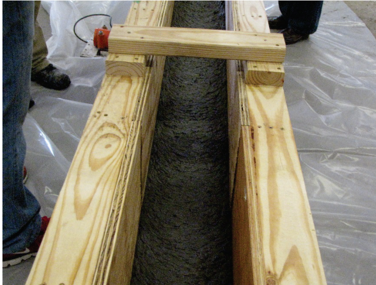
Figure 3.3. Formation of “skin” during casting.
