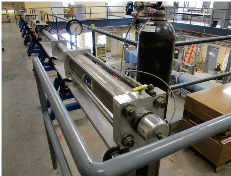
Figure 3.12. SHPB instrument looking toward output bar. The compressed nitrogen cannon is in the foreground.
