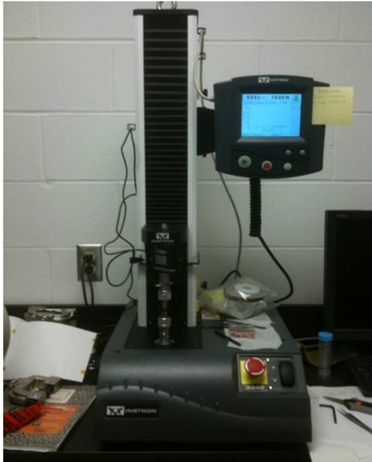
Figure 2-5. Optical image of Instron column used to measure stress vs. strain curves.
