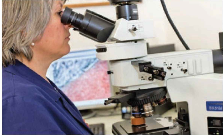
The microstructure of a steel is checked under high magnification. Photo: Acroni, Jesenice (SI)
