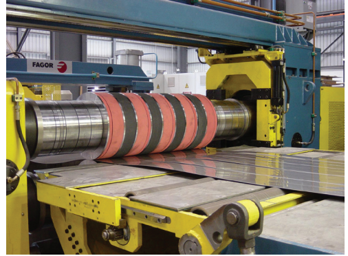
Photo 3: Slitting line in action
