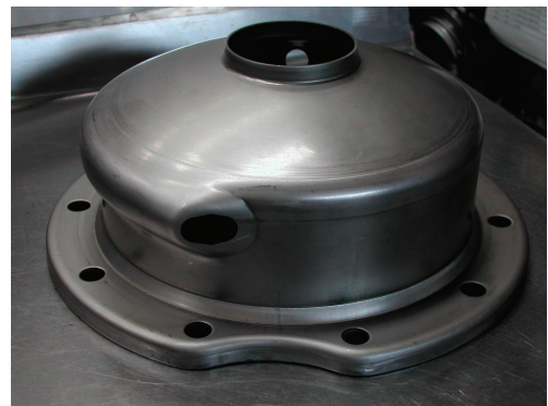
Photo 16: Pump casing: the high ductility of austenitic stainless steels makes them suitable for one-piece designs combining deepdrawing and hydroforming techniques.
