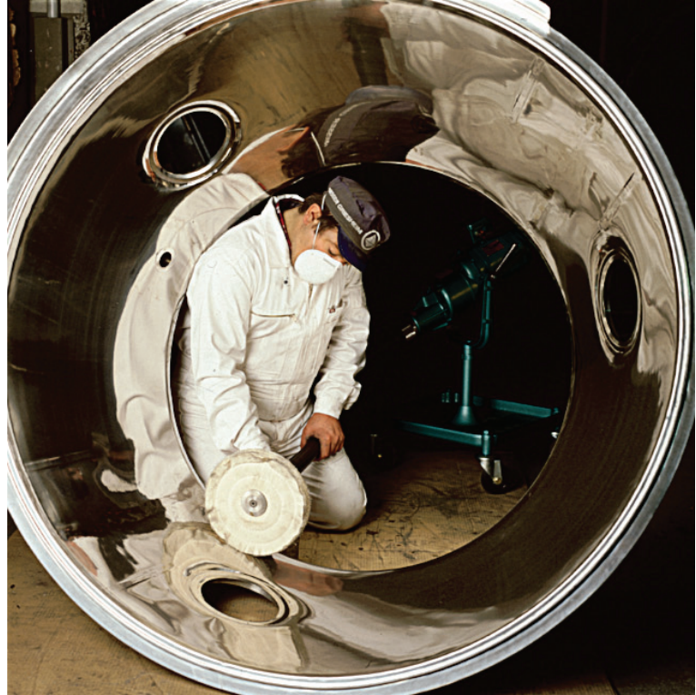
Photo 12: Surface finishing. A variety of different finishes – such as mirror polish – can be achieved to meet technical requirements
