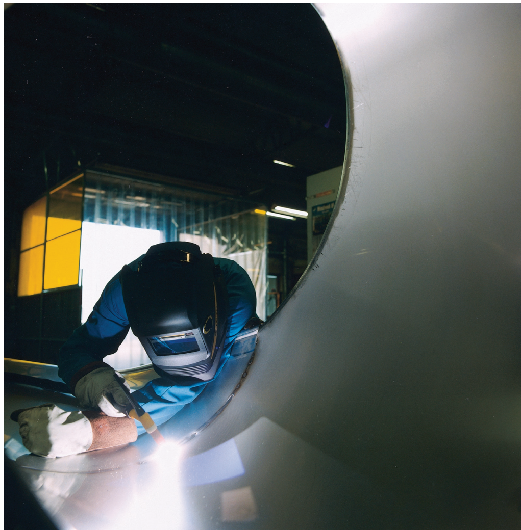
Photo 9: Manual Gas Tungsten Arc Welding
