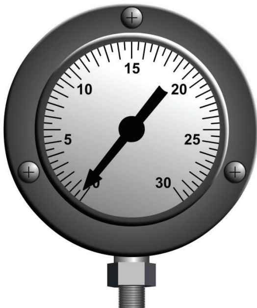
Figure 8-4 — Bourdon-tube vacuum gauge.
