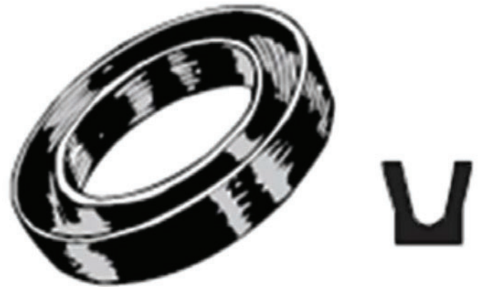
Figure 7-22 — Typical U-cup seal.
