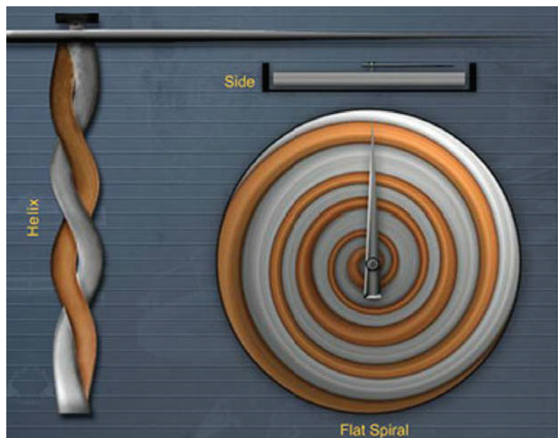
Figure 8-12 — Bimetallic thermometer (flat, spiral strip).
