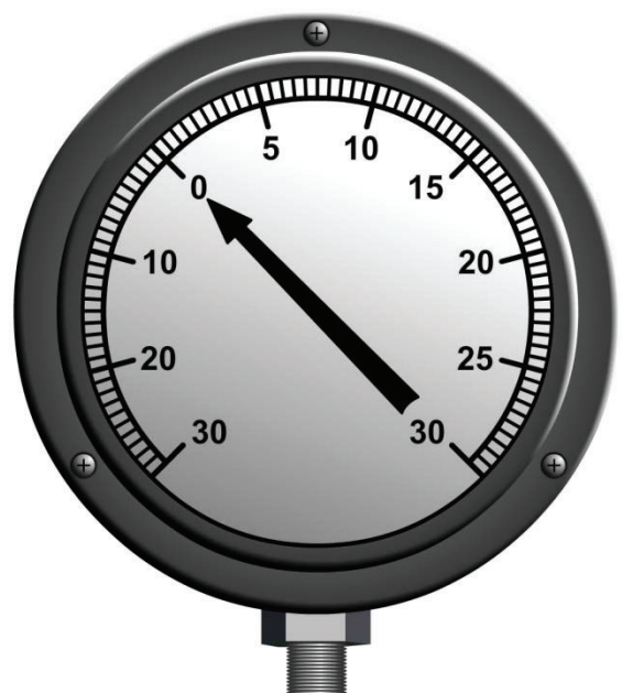
Figure 8-5 — Compound Bourdon-tube gauge.
