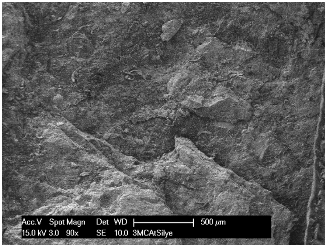
Figure B13. Photomicrograph of the exterior surface from the supply pipe of the fire suppression system at Chimyu-Wan fuel storage, Okinawa, Japan. (90x)
