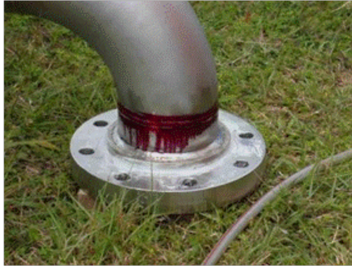
Figure 5. DPT application for nondestructive testing of welds.
