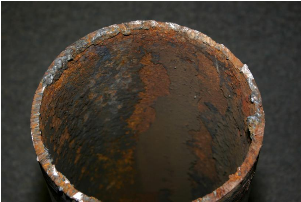
Figure B9. Photograph of the interior of the pipe as received from Okinawa showing light general corrosion.
