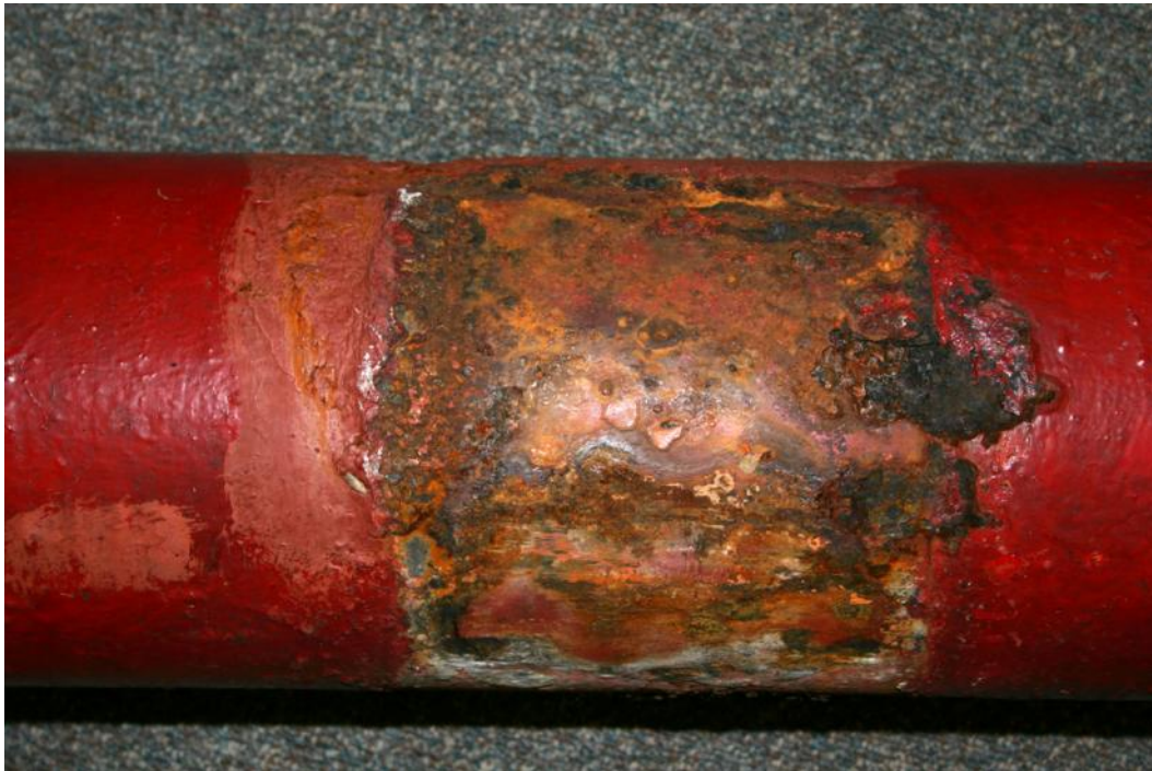
Figure B7. Photograph of the area of the pipe in contact with the concrete saddle in the field.
