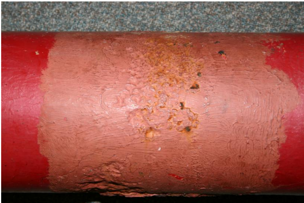
Figure B8. Photograph of the pipe section showing the area under the strap used to hold the pipe to the saddle.
