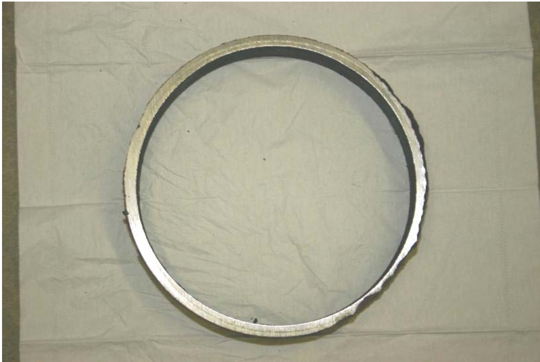
Figure B11. Photograph of the cross section of the pipe showing the wall thinning near the area of the support saddle.
