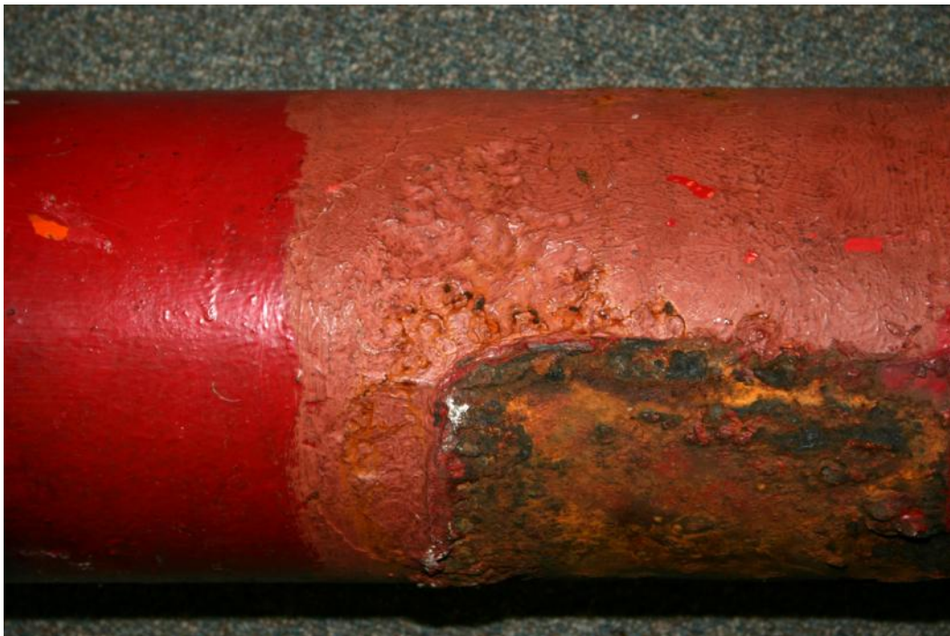
Figure B6. Photograph of the pipe section as received from Okinawa showing the area near and under the support saddle.
