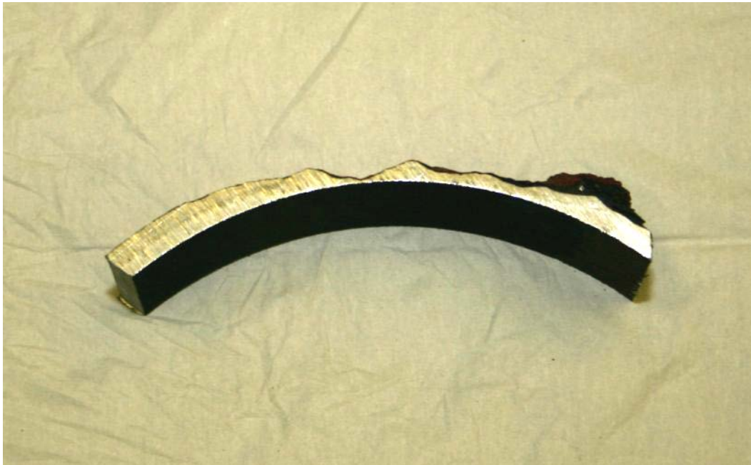
Figure B12. Photograph of the deeply corroded area on the outside of the pipe.
