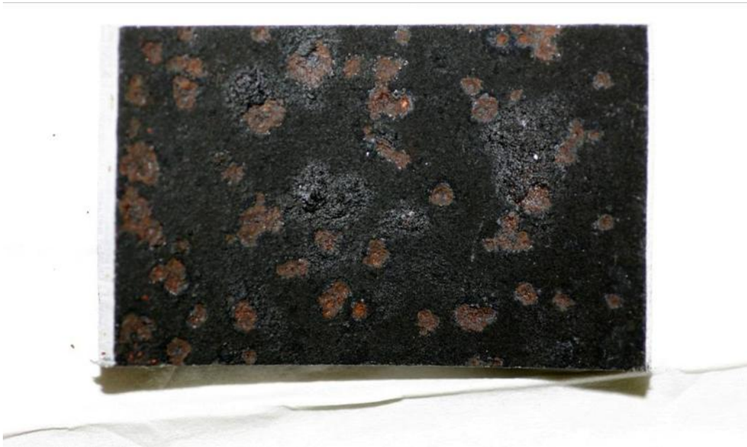
Figure B10. Photograph of the interior of the pipe showing the beginning of pitting corrosion from the water carried in the pipe.
