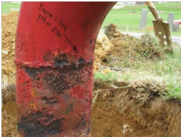
Figure 3. Severe pitting on above-grade riser.
