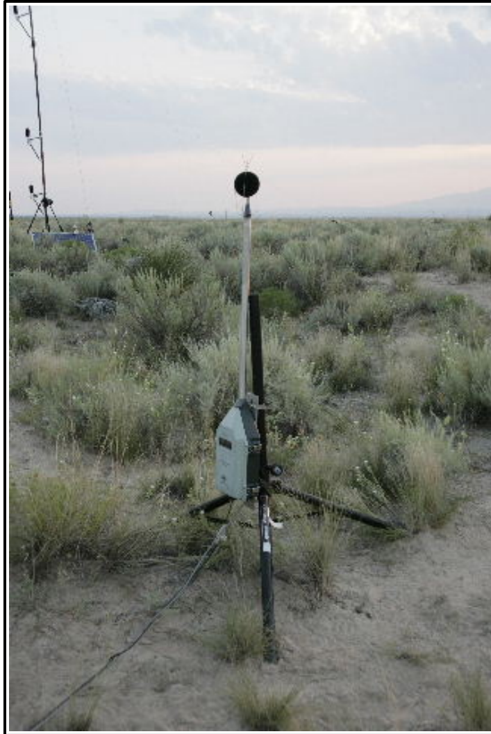
Figure 2-2. Representative remote acoustical measurement station.
