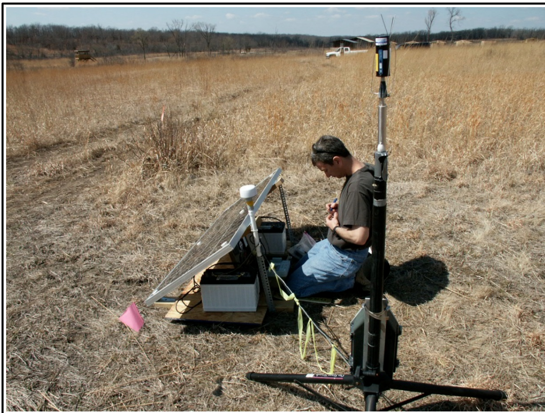
Figure 2-4. Calibration procedure in process. (The calibrator is the black cylinder placed on top of the tripod.)
