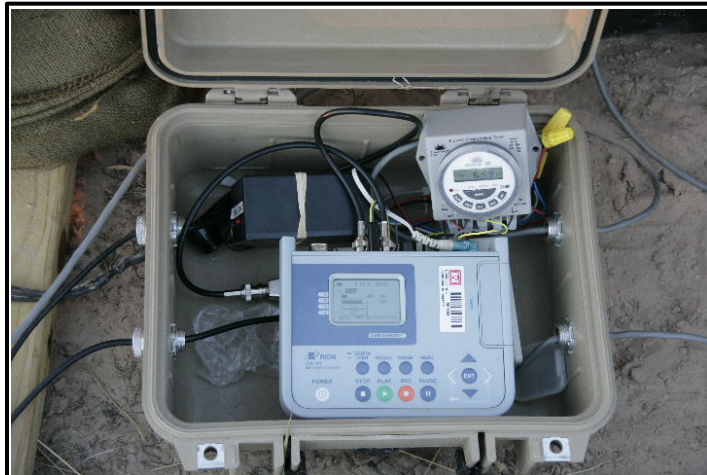
Figure 2-3. Representative instrumentation box for remote acoustical measurement station.
