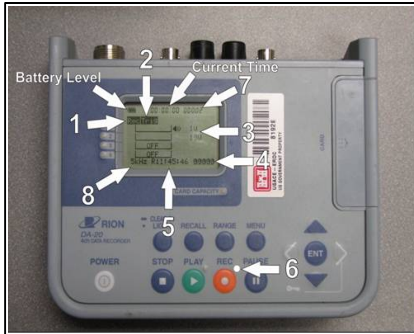
Figure 2-6. A RION unit that has been properly setup and is ready to begin collecting data.
