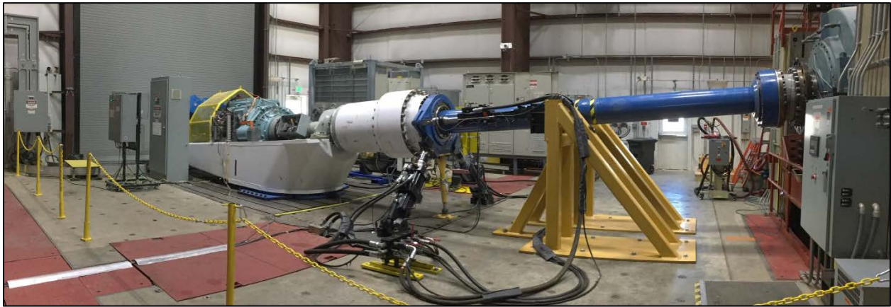
Figure 4. Drivetrain dynamometer installation. Photo by Jonathan Keller, NREL 40428
