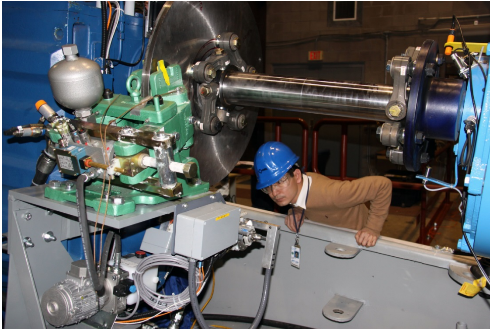
Figure 17. GRC braking system hardware. Photo by Joe Verrengia, NREL 16867
