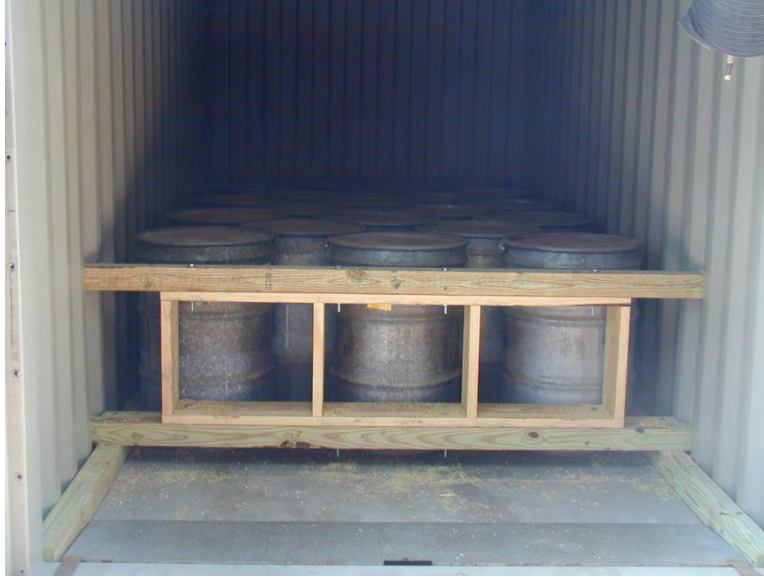
Figure 7-3. Drums that are properly blocked and braced
