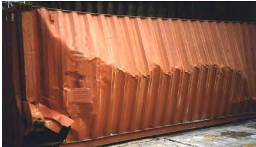
Figure 7-1. Damaged Freight Container from Internal Contents
