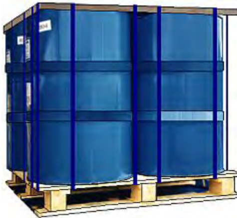
Figure 7-4. Properly palletized drums
