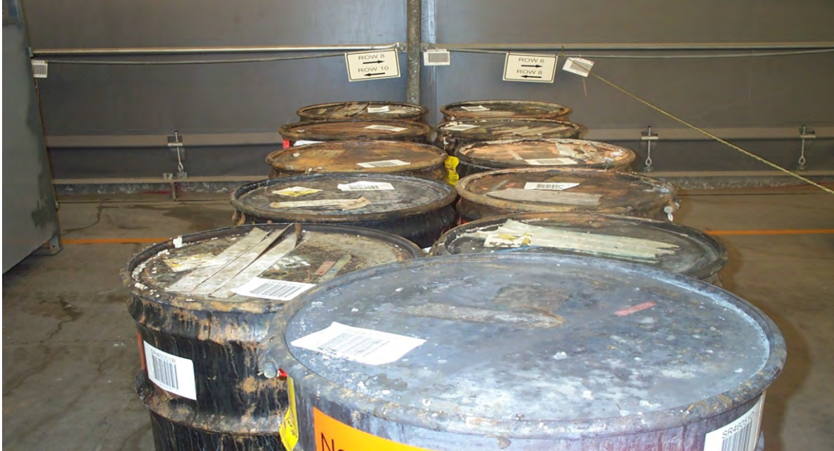
Figure 4-1. Degraded packagings with dispersible contents inside or packagings with external contamination are considered dispersible contents.
