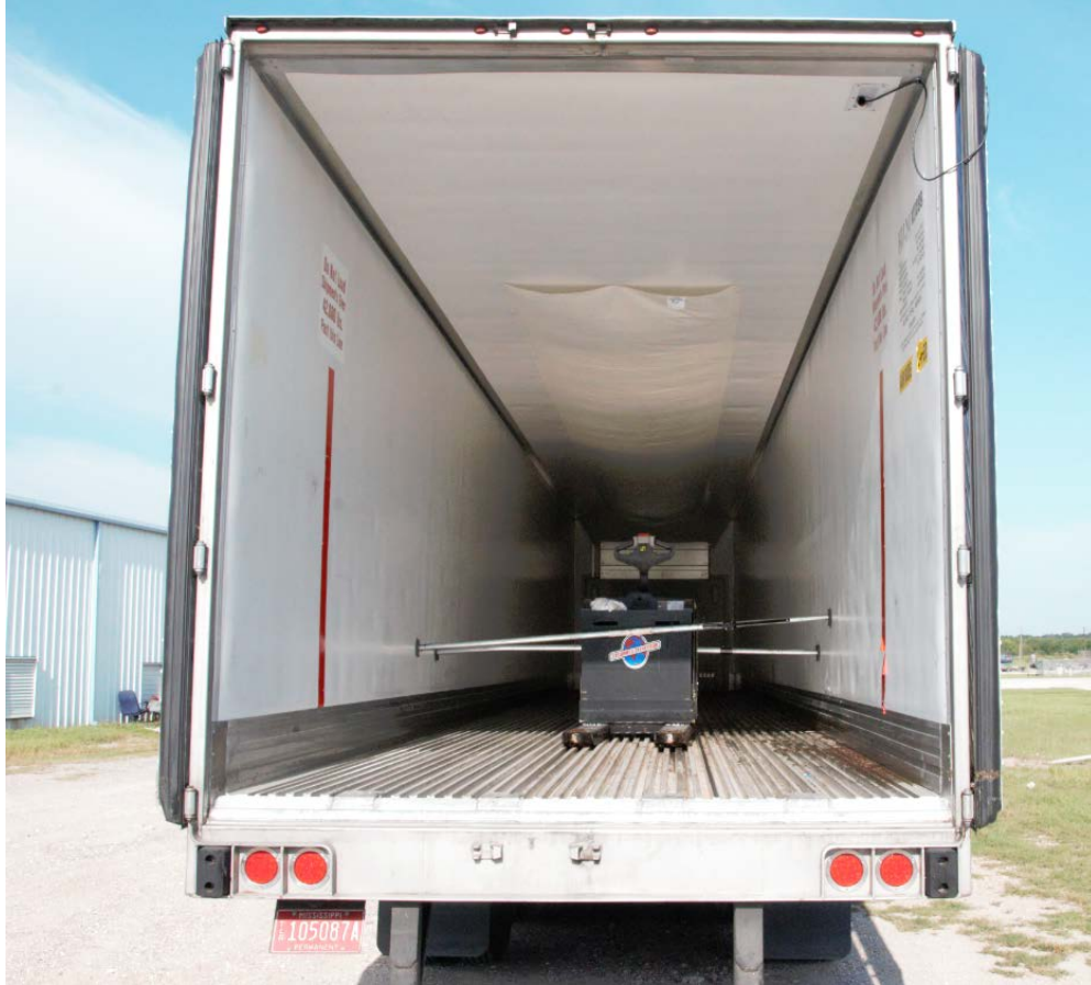
Figure 7. Refrigerated Truck Trailer. Arkema used about a dozen refrigerated truck trailers like this one used to ship organic peroxide products to customers and to provide a temporary storage location if the refrigeration at one or more of the Low Temperature Warehouses could not be maintained. (Source: CSB Photo)
