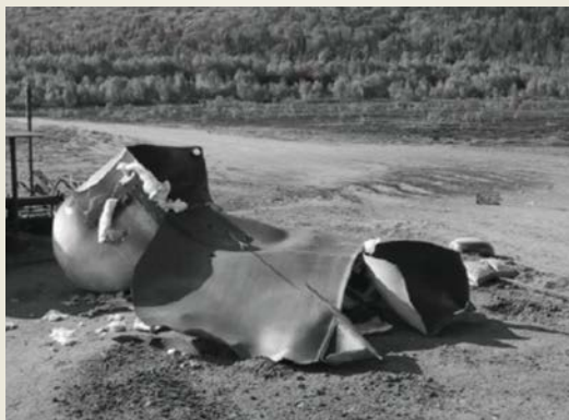
Vessel flattened on ground following BLEVE. iii
