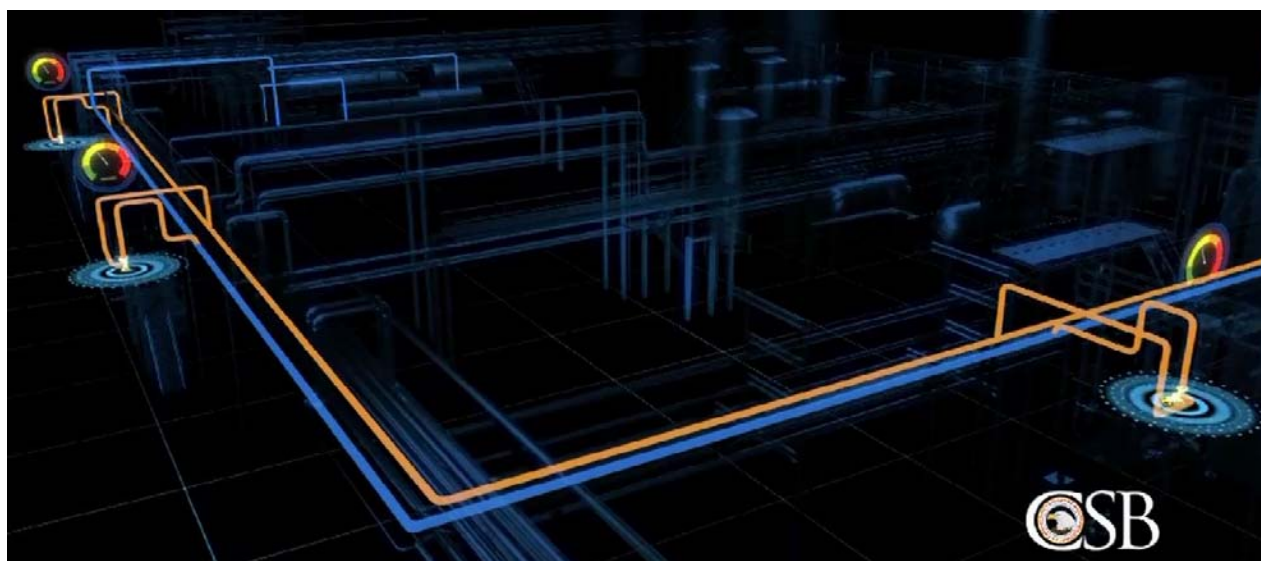
Figure 31. Excerpt from CSB Animation. It depicts the three locations where valves connected the methyl mercaptan feed piping (blue) to the waste gas vent header piping (orange). Workers used the pressure gauges shown at these locations to monitor the progress of clearing the hydrate blockage inside the methyl mercaptan feed piping. Source: CSB.
